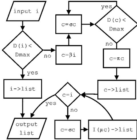
FIG. 3. The MAXDEEP algorithm that finds stitches with depths below  $D_{\max}$ . For a given input node  $i$ , it returns a list of those nodes in  $\Delta(i)$  that fulfill the criterion in Eq. (15).  $c$  is the tree climber,  $\rightarrow$  means push (i.e., “put on a list”), and  $I(\mu c)$  is the output of a recursive call to the algorithm itself with  $\mu c$  as the input node. The diagram can be read in conjunction with Fig. 2.
